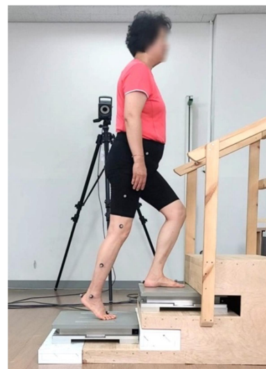
Figure 1. Staircase structure used for gait assessment. The structure consisted of three steps, each 18 cm in height. Ground reaction forces and COP were measured using a force plate embedded in the second step. Participants performed stair ascent and descent barefoot, starting with the dominant leg at a self-selected speed.
